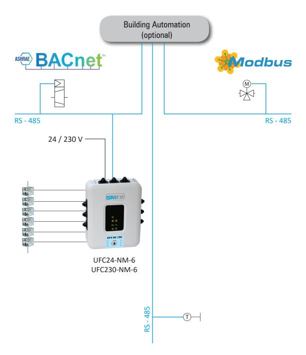
Upon request, SMT supplies the functional profile of the UFC devices for the easy integration into any Modbus or BACnet controller
