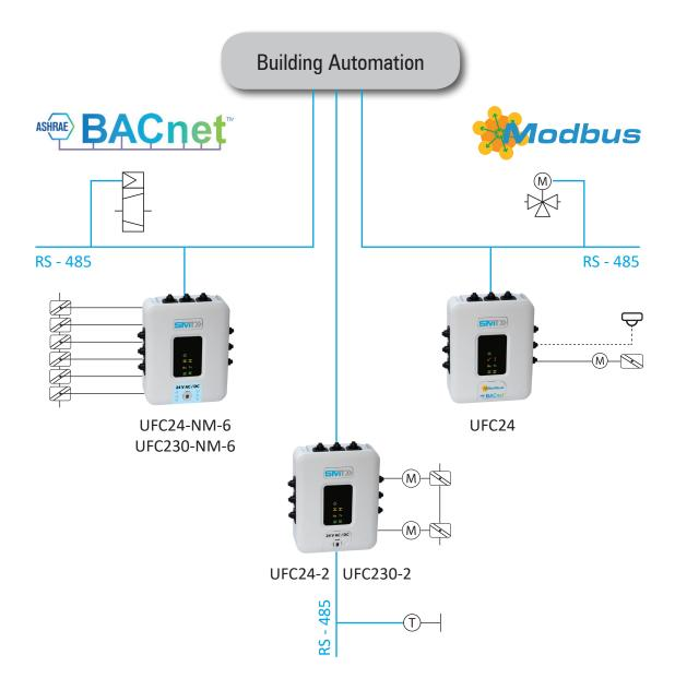
Upon request, SMT supplies the functional profile of the UFC devices for the easy integration into any Modbus or BACnet controller
