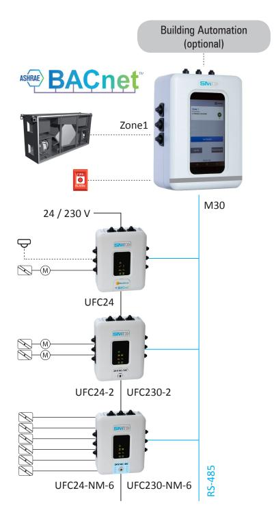
Individual control of 2 dampers together with the UFC24-2 / UFC230-2
